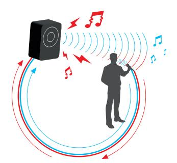
The common method employed by sound engineers to limit Larsen effect is to manually equalize the frequency response of the sound reinforcement system, and to limit the gain of the microphone. But there are also systems that automatically limit the feedback effect.
